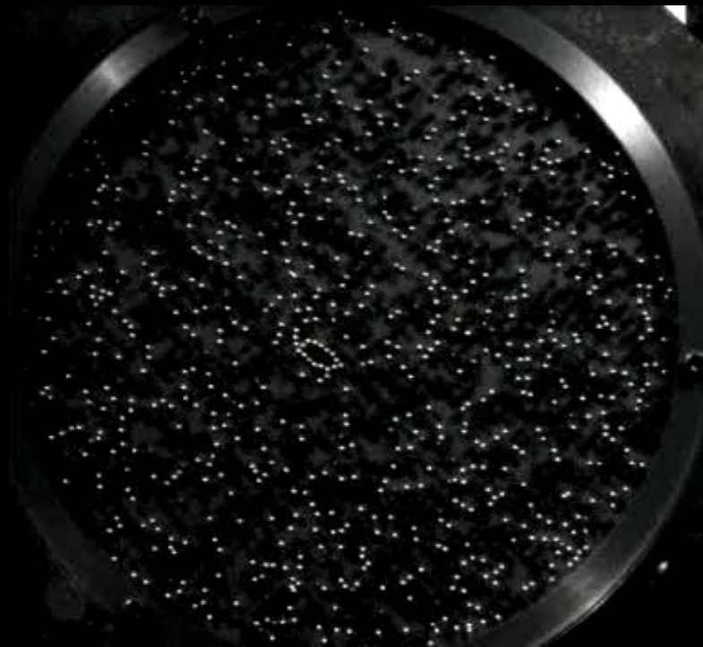
Clustering of dipolar magnetized particles in a vibrated container (from A. Kudrolli's group)
